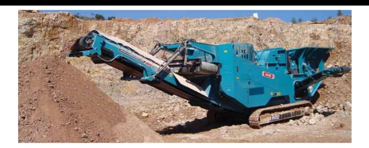
The Powerscreen® XH250 horizontal shaft impactor is a compact track mobile crusher designed for small to medium sized operators in the recycling and demolition markets. Capable of processing a wide range of material at a high output, the plant is versatile, easy to operate and fuel efficient due to its direct drive system.
