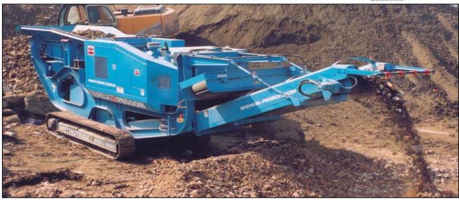
Above image features a Metrotrak fitted with the optional side conveyor and overband magnetic separator
