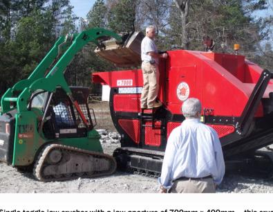
Description: Single toggle jaw crusher with a jaw aperture of 700mm x 400mm – this crusher will crush a full UK kerbstone in approximately 10 seconds. The 7000 series is 2200mm wide and a has a loading height of 2720mm. This machine will provide significant daily tonnage where a larger machines is too bulky or noisy. The 7000 series will produce an output size ranging from 20mm up to 120mm.
