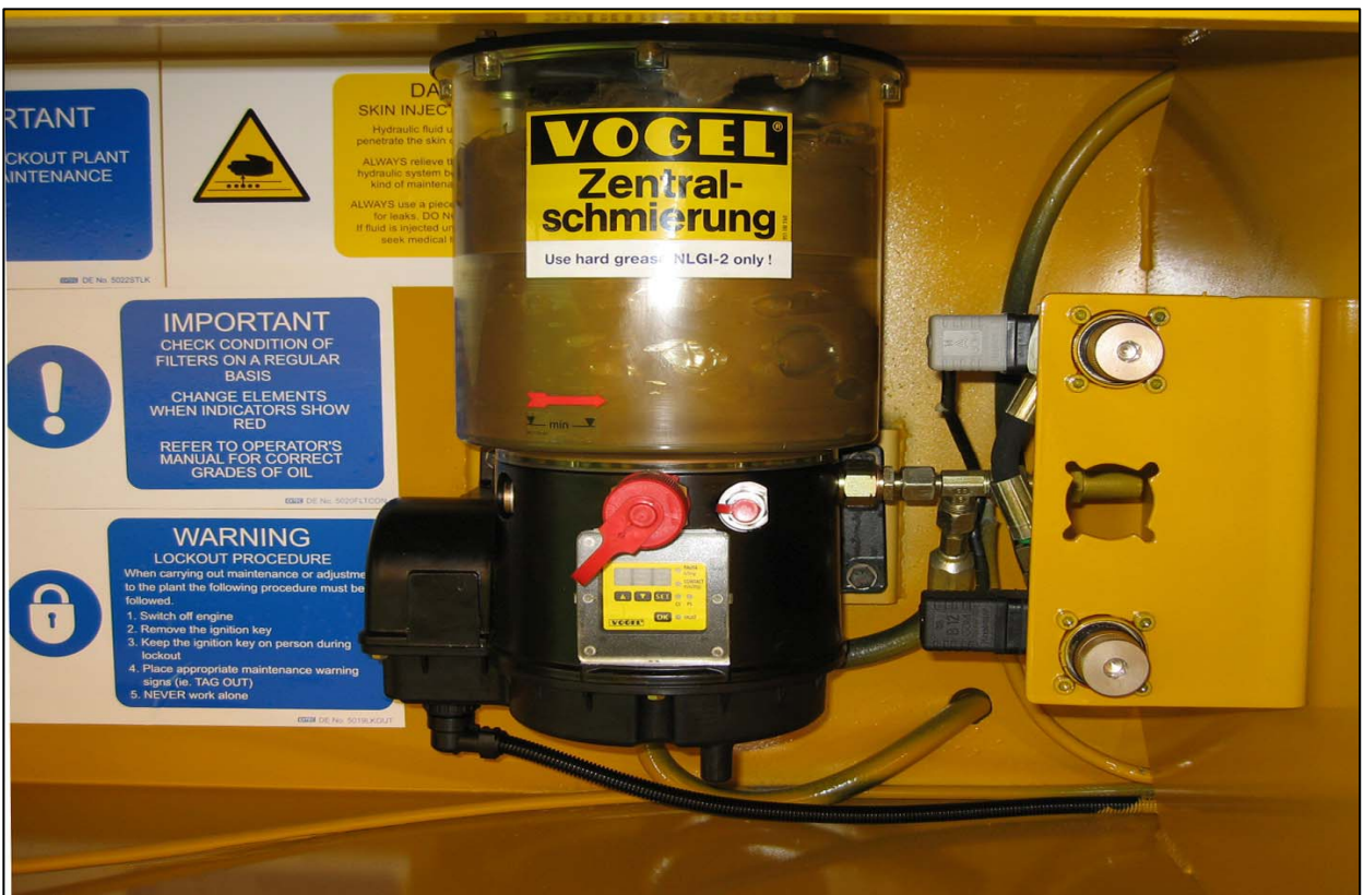
SKF automatic lubrication – reduced wear and downtime
