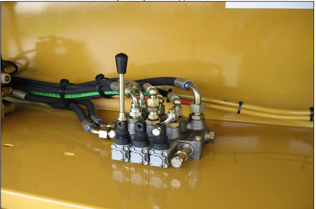
Extended main conveyor control
