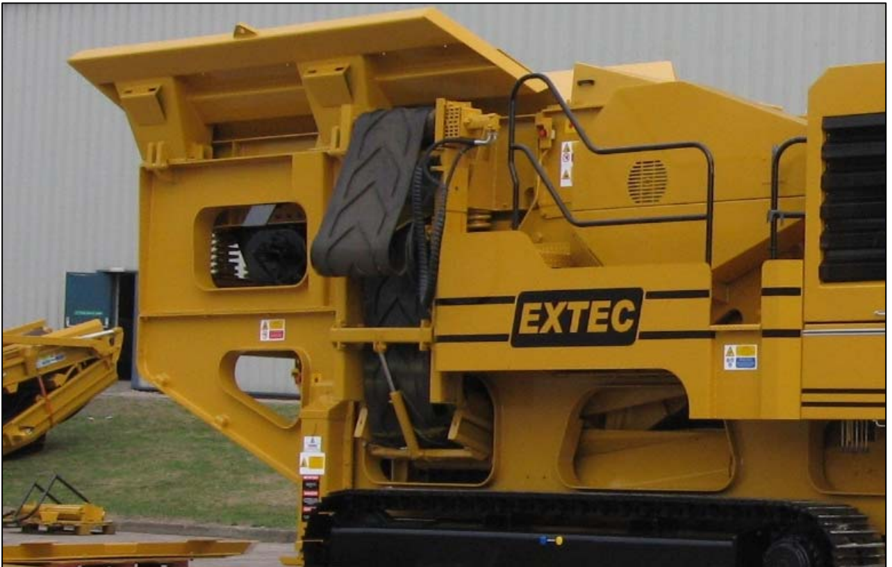
New Heavy Steel, Web and Flange Frame Construction
