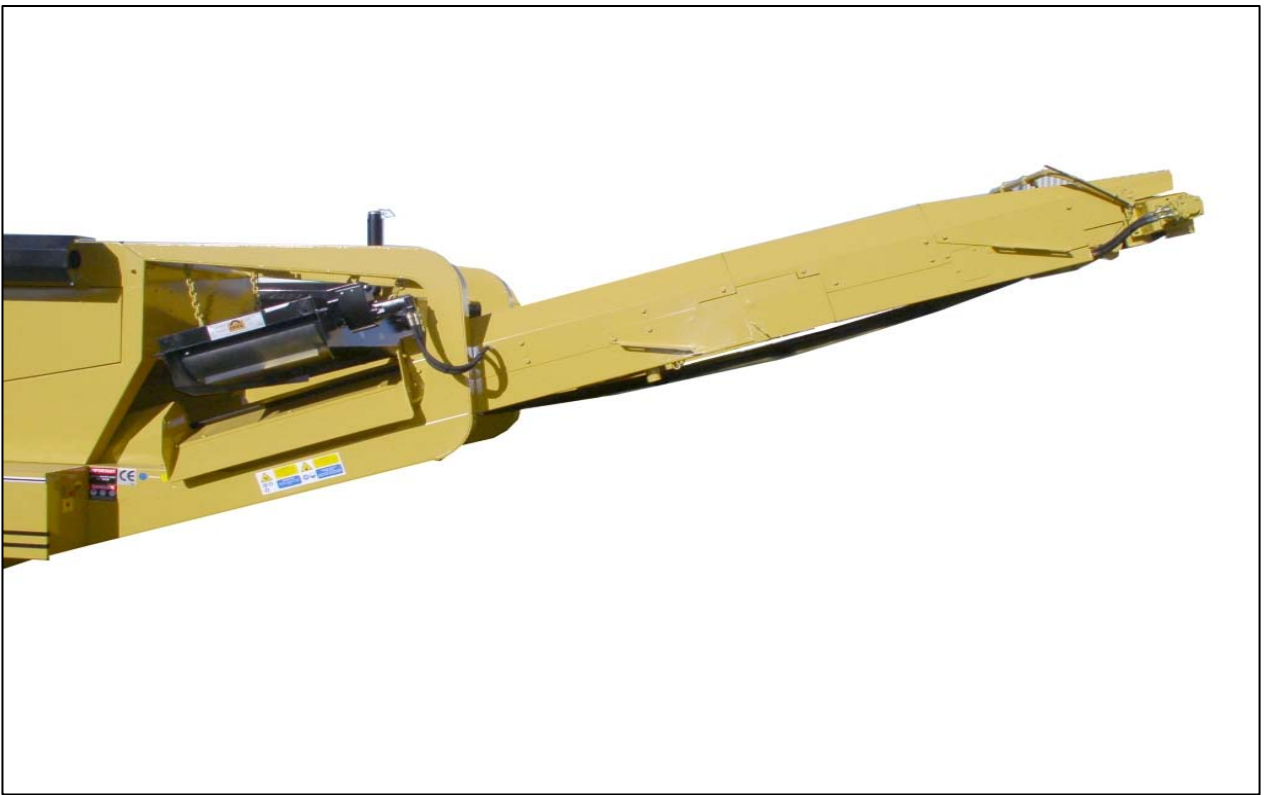
Extended main conveyor- no need for ramps for onward machine feeding and stock piles
