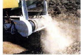
The MC140P is based on our technology used in our NC Automobal series. The MC140P is equipped with reciprocating plate feeder and AC jaw crusher on the undercarriage. Best suited mini jaw crusher for small-scale demolition sites.
