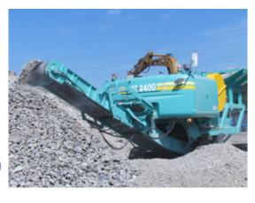
The MC240G is fully equipped with features such as grizzly feeder, automatic feed control system, overload protection device, and a powerful 55PS diesel engine that enhance its performance and make the maintenance easy. It is the most efficient, full-spec crawler mounted jaw crusher in this size range.
